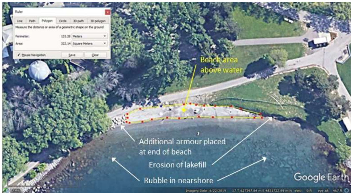
Figure 2.5: Narrow south shore (beach area above water approximately 320 m 2 ); additional armour placed at west end; erosion of lakefill at east side; and rubble in nearshore (ref. Google Earth 2019/6/22)
